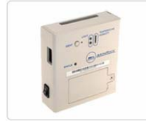
Fig. 2 Arch Rock IP sensor node
