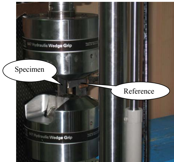
Fig. 3 Specimen mounting details for IRT test
