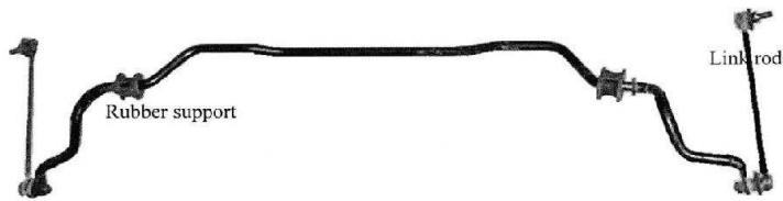
Fig. 2 The picture of the undamaged anti-roll bar analysed in this study
