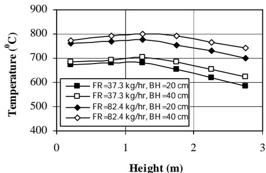
Fig. 2 Effects of the combustor loading and bed height on the axial temperature profiles in the conical FBC for the tests conducted at quasi-identical EA of 59-63%
