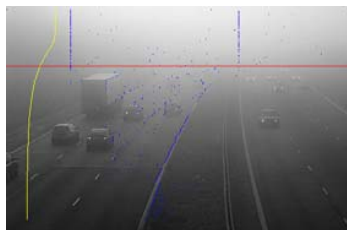
Fig. 8 Daytime fog detection and computation of the meteorological visibility distance (red line)
