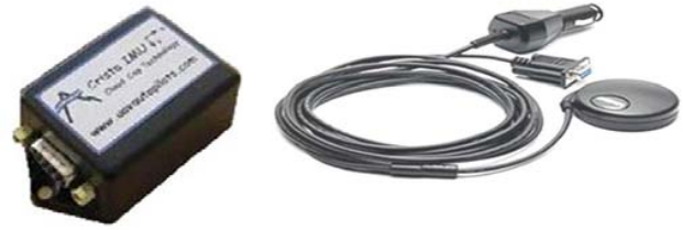
Fig. 8. The cloud cap technology Crista IMU which is a very small, low-cost, 3-axis MEMS inertial measurement unit (left). GPS 18 PC with DB-9 pin serial connector (right).
