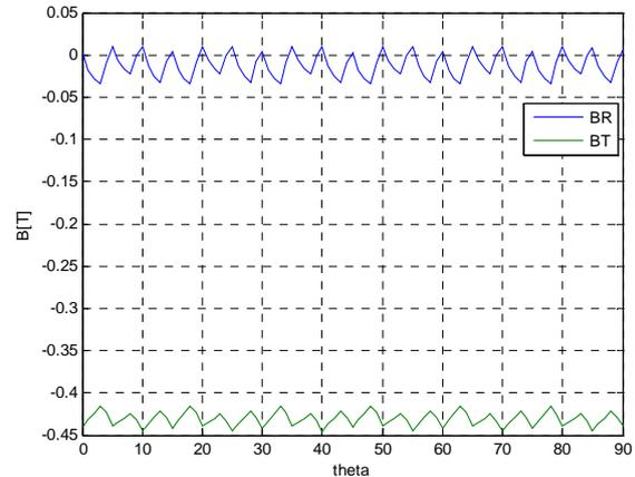
Fig. 2 Radial and tangential components ( $B_R$ ,  $B_T$ ) on magnet obtained with 2D-FE, versus rotor position mechanical angle.
