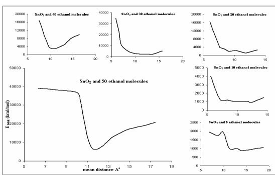
Fig. 4 The total energy (kcal/mol) calculated for interaction  $\text{SnO}_2$  and ethanol molecules in different mean distance ( $\text{\AA}$ ) at 298K by Langevin Dynamin simulation
