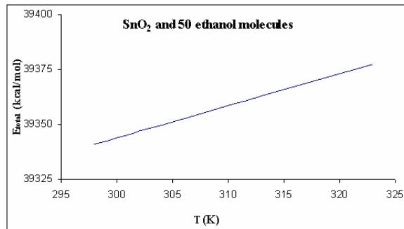
Fig. 3 The total energy (kcal/mol) calculated for interaction  $SnO_2$  and ethanol in mean distance  $6.31\text{ \AA}^{\circ}$  and different temperatures by Langevin Dynamin simulation
