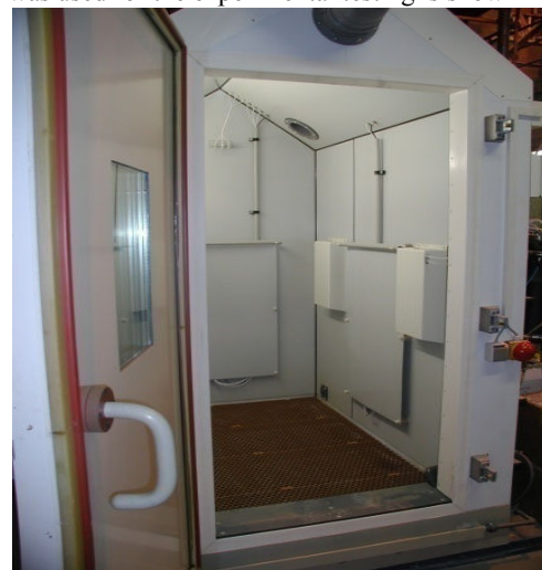
Fig. 2 KWT4300 Walk in salt fog chamber
