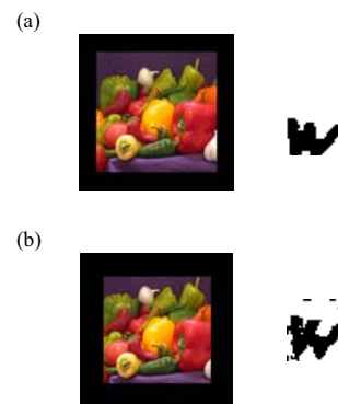
Fig.6 (a) Watermarked image cropped by 226 \times 226 mask along with its extracted watermark, (b) Watermarked image cropped by 216 \times 216 mask along with its extracted watermark
