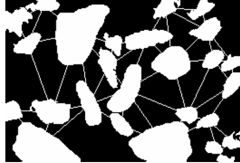
Fig. 15 Inter-particle distance analysis on lab compacted HMA cross-sectional slice
