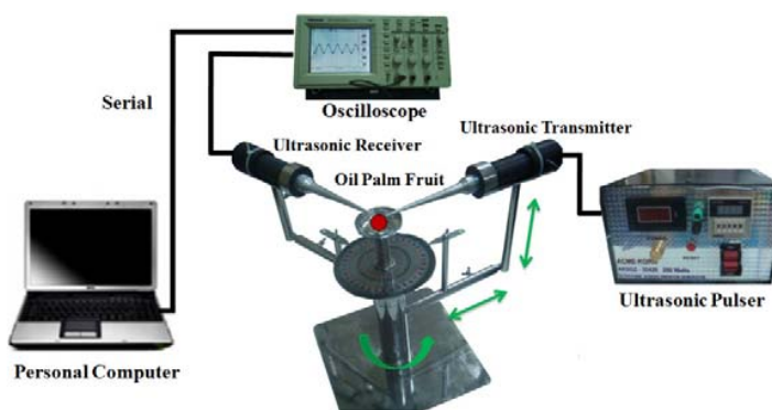
Fig. 1 Ultrasonic experimental setup
