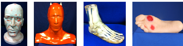
Fig. 1 The four anatomical phantoms used in this investigation (a) polystyrene head mannequin model; (b) plastic radiography head model with 12 traverse slices; (c) a Perspex foot with bone encapsulated; (d) silicone based foot with 3 simulated ulcers
