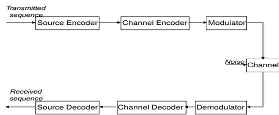
Fig. 1. Communication system model
