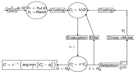
Fig. 2 Decoding of Linear Block Codes based genetic algorithm
