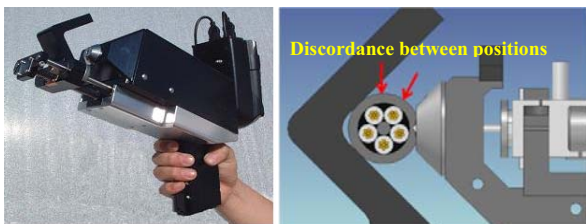
Fig. 3 Cable indenter by KEPRI and its occurred discordanace
