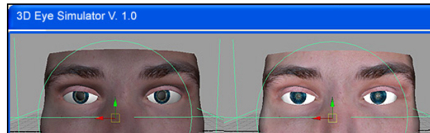
Fig. 4 Change in "light_intensity" parameter with consequent change in pupil size. "Light_intensity" = -5 on the left; "Light_intensity" = +5 on the right
