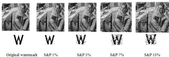
Fig. 14 Stego image and Extracted watermark after different Salt and Pepper percentages images
