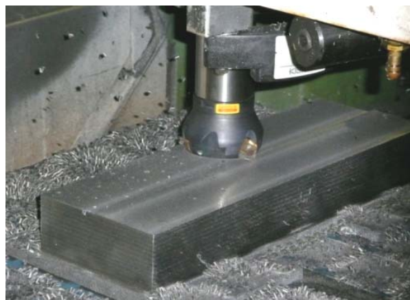
Fig. 2 Magnetic clamping of the workpieces
