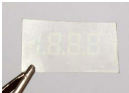
Fig. 5 Photo of the real structure, patterned by photolithographical process on the polymer sheet
