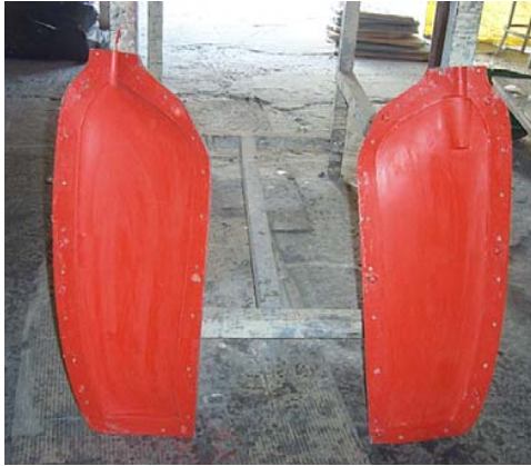
Fig. 14 Inside of the mold made of glass fiber
