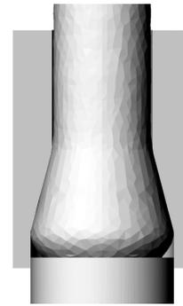
Fig.3 Pipe Buckling
