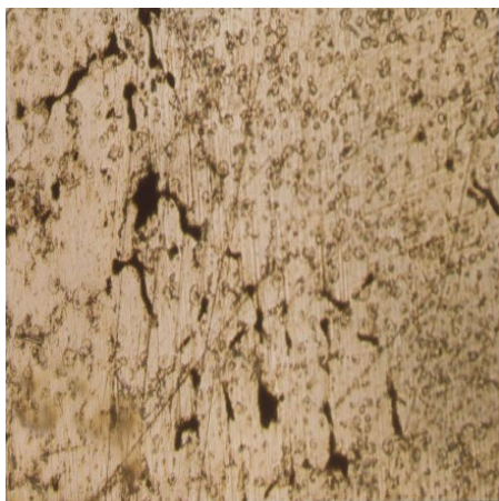
Fig. 4 Microstructure of Al-Zn-Mg Alloy Sample (Ageing 95 days at Room Temperature), 100X
