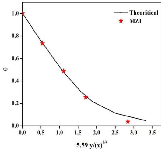
Fig. 4 Comparison of the temperature distribution in the vicinity of a heated surface, obtained using MZI with theoretical [14]
