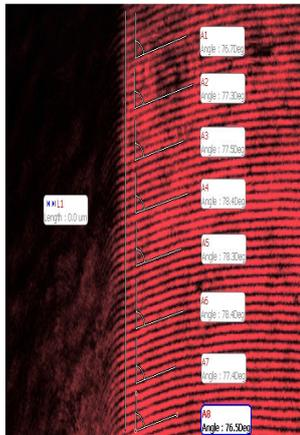
Fig. 5 Typical Interferogram obtained for a surface temperature of 40°C. The bending angles are marked in the figure
