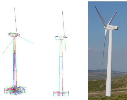
Fig. 3 Wireframe model and photo of the wind turbine MADE AE-46/1
