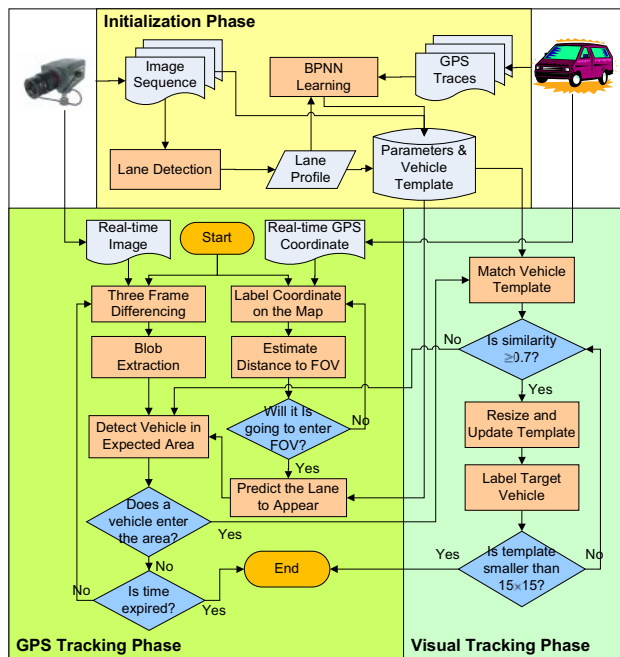
Fig. 3 The operation process of GPS-VT for vehicles
