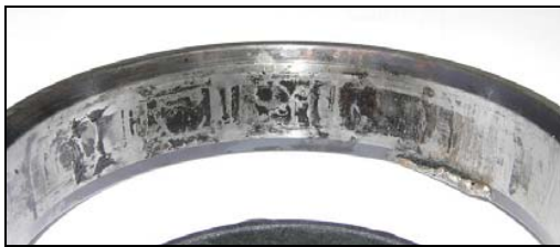
Fig. 14 The defects (dark marks) in the outer race of the bearing
