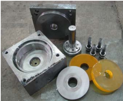
Fig. 2 Photograph of the new die set parts
