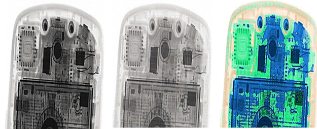
Fig. 1 Production of color encoded image from (a) Low energy image, (b) High energy image and (c) Color encoded X-ray image
