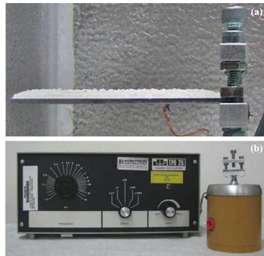
Fig. 4 (a) Lateral view of the clamped ice-aluminum composite beam and (b) Electro-magnetic shaker system
