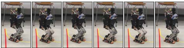
Fig. 8. The experiments for the biped robot tracking to curved path
