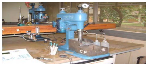
Fig. 4 Laboratory flotation machine, Denver D 12
