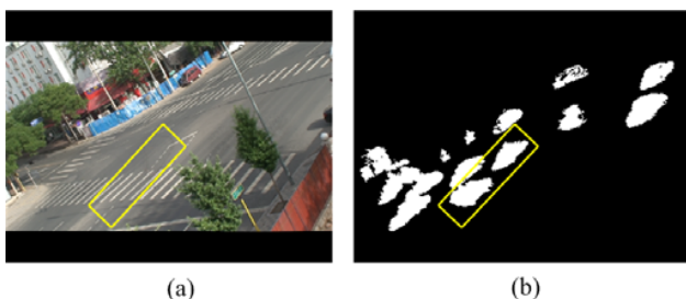
Fig. 7 Vehicle-vehicle traffic conflict detected by improved algorithm: (a) subtracted background; and (b) extracted moving objects
