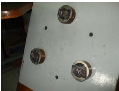
Fig. 2 The arrangement of the specimen holders and test pieces attached underneath the sled
