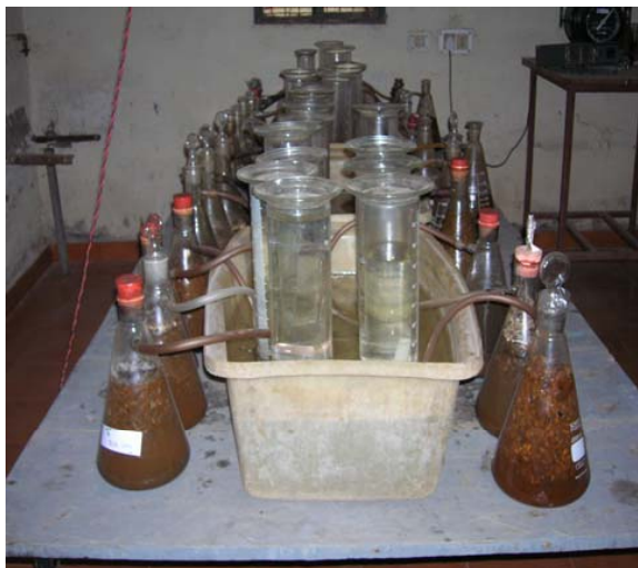
Fig. 1 Experimental set up for biogas production
