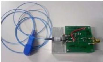
Fig.2 Configuration of ROSA PIN-PD with Pre-Amplifier
