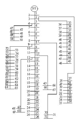
Fig. 1. 69-bus radial distribution system
