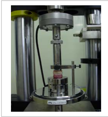
Fig. 4 Configuration of the compressive test using Instron Microtest System (5848 series, Instron, Norwood, MA, USA)
