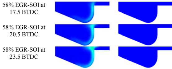
Fig. 16b Contour plots of soot (left) and NOx (right) mass fraction at different SOI at 360 °CA
