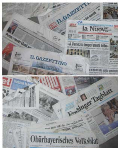
Fig. 1. Visually flexo-printed newspapers (top) and offset-printed newspapers (bottom) are hardly distinguishable. Even experts can identify flexo-printed only by the newspaper title (e.g. Daily Mail, Il Gazzettino) or a magnifying glass. NIR spectral imaging identifies flexo-printed newspapers in real-time and thus enables the development of industrial sorting systems.
