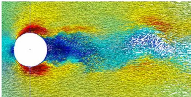
Fig. 8 Instantaneous velocity vectors close up view from the top for  $R=5000$ . Scale starts from 2.256 for the red color.
