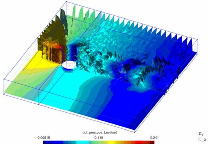
Fig.7 Pressure instantaneous isosurfaces for R=5000
