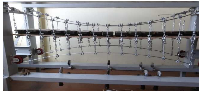
Fig. 11 Model of single cable top chord
