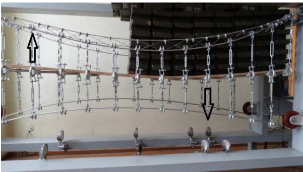
Fig. 23 Displacements in non-symmetrical loading case
