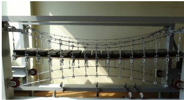
Fig. 12 Model of cable truss top chord
