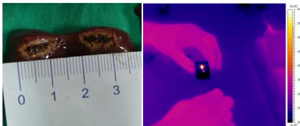
Fig. 3 Measure of damage volume and infrared thermography
