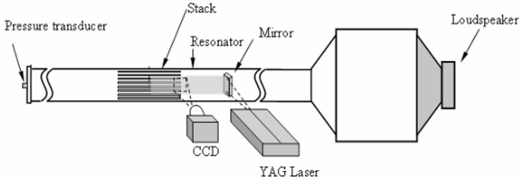
Fig. 1 Sketch of the experimental apparatus
