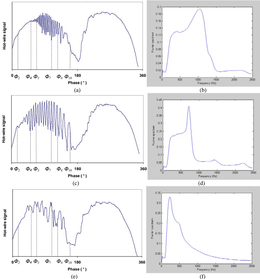
Fig. 7 Hot-wire signal traces within an acoustic cycle and the corresponding frequency spectrum; a, b ( $d = 0.5\text{mm}$ ,  $D = 4.8\text{mm}$ ,  $Re_d = 207$ ,  $Dr = 2.0\%$ ); c, d ( $d = 1\text{mm}$ ,  $D = 4.8\text{mm}$ ,  $Re_d = 433$ ,  $Dr = 2.0\%$ ); e, f ( $d = 4\text{mm}$ ,  $D = 9.6\text{mm}$ ,  $Re_d = 1395$ ,  $Dr = 1.5\%$ )
