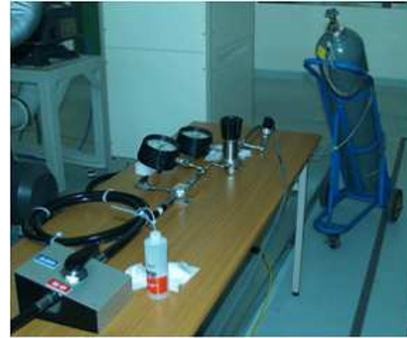
Fig. 7 High pressure nitrogen tank and propellant supply line
