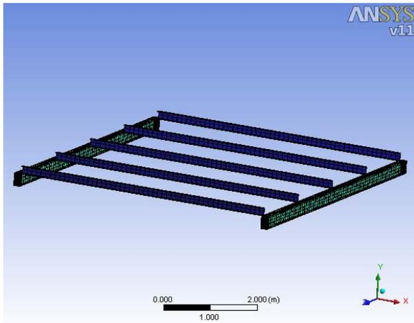
Fig. 5 The geometry of system with purlins
