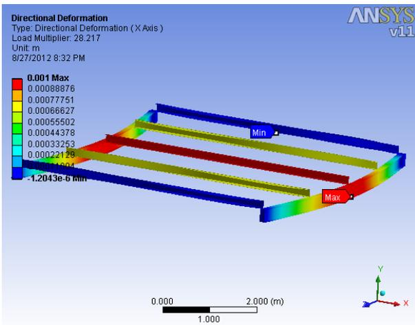
Fig. 13 The buckling mode for column with purlins (single mode)
