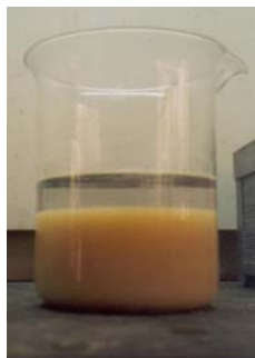
Figure (3) Precipitation of rare earth hydroxide
