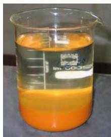
Figure (7) Precipitation of Cerium Hydroxide after solvent extraction process
