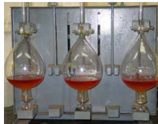
Figure (5) Extraction with TBP
