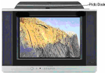
Fig. 5 Position of Photo Diode
