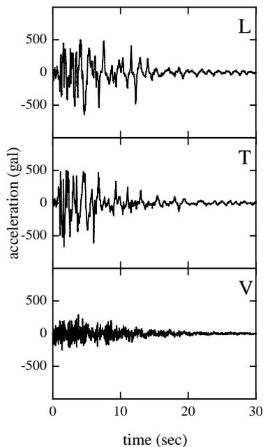
Fig. 4 JR Takatori St. Record, 1995 Kobe Earthquake.
