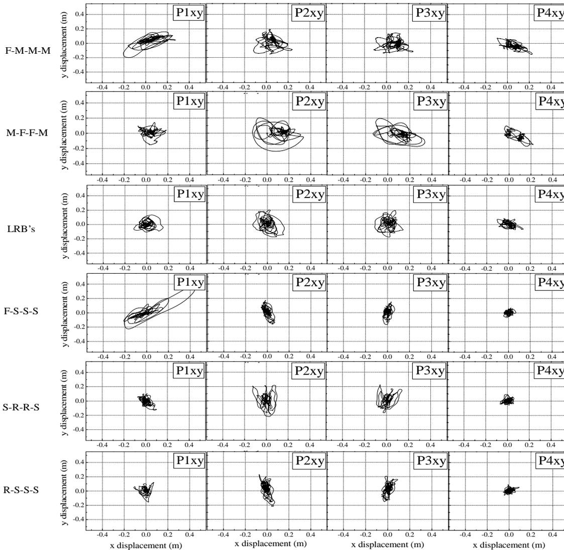
Fig. 9 Pier top displacement trajectories
