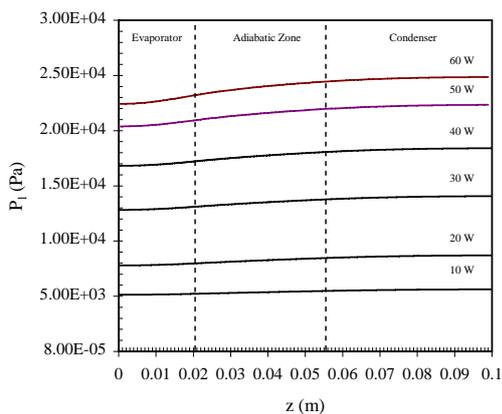
Fig. 21. Variations of the liquid pressure  $P_l$
