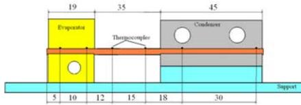
Fig. 5. Thermocouple locations
