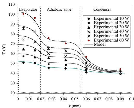
Fig. 24. Variations of the FMHP wall temperature
