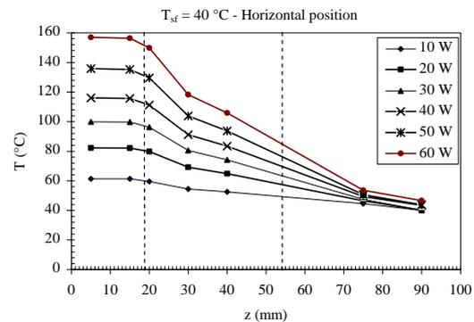
Fig. 8. Copper plate axial temperature profile
