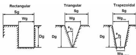
Fig. 2. Geometrical parameters of the groove shapes
