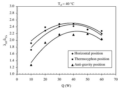
Fig. 14. Effective thermal conductivity enhancement variations as a function of Q, for different orientations ( $T_{sf} = 40^{\circ}\text{C}$ )
