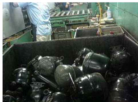
Fig. 6 Compressors Divided from Waste Home Appliances
